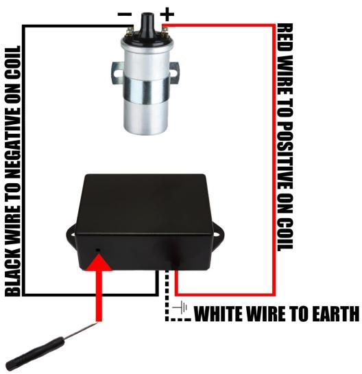
Once wired tick-over on car should be increased, for initial setup, to around 3000 RPM on a 4 cyl cars. for 6 & 8 cyl will need to be 4000RPM. The adjustment screw should now be adjusted until the engine slows or misfire. This is a soft cut limiter so the engine will NOT stop.
